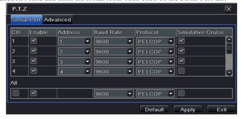
Chose the channel that the PTZ camera is connected to and make sure the Enable check box is checked. Set the address of the PTZ camera (usually defaults to 1). Set the Baud Rate to 2400. Set the Protocol to PelcoP. Click the Apply button to save the changes and then Exit. Right-click on the main screen and select P.T.Z camera option. This will bring up a PTZ control window and you should be able to control the camera (as long as all of the wiring is correct.).
